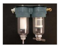
The dual filter includes an automatic drain and a power drain with a valve that works as a check valve. It runs pressure through the orifice and is a Venturi, drawing the moisture out from the bowl under pressure, dispelling the moisture, and disallowing any air to come up into the bowl. This prevents water and contaminants from coming through the pump. This filter provides good service and good reliability for your pump.
